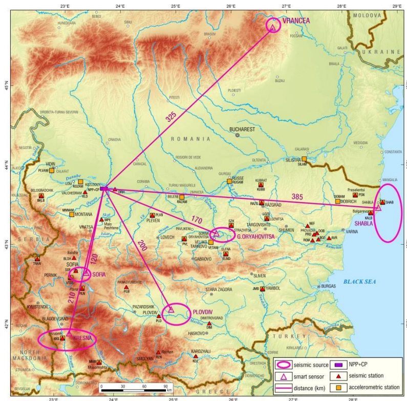
Fig. 3. Schematic map of the main seismic sources, distances to the NPP Kozloduy, smart sensors locations and the seismic network.
