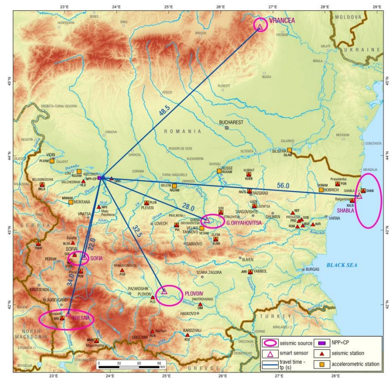
Fig. 4. Schematic map of the main seismic sources, smart sensors locations, the seismic network and travel times of P waves ( t_p ) – data from Table 2.
